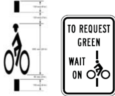
OMUTCD approved bicycle detection marking and signage.
