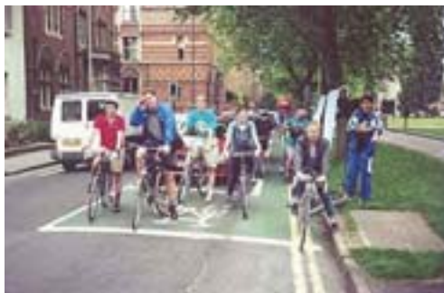
Bicycle Box in England filled in with color to emphasize allocation of space to bicycle traffic.
