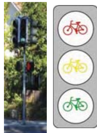
Bicycle traffic signal.
